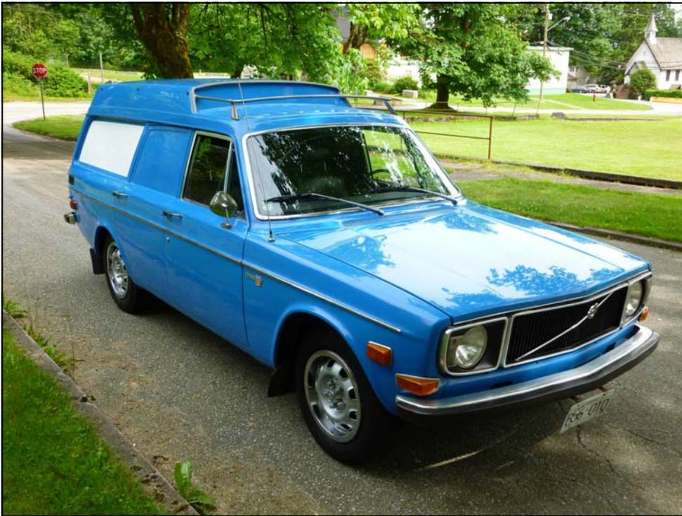
glass but carried the standard rear window glass and opened upwards like all 145 wagons, only much higher. Inside there were no rear seats and a cargo screen was fitted just behind the front seat line. Wooden slats protected the sides and deck of the cargo area. The rear passenger doors were fitted and functional but had sheet metal in place of windows. The cargo area also had sheet metal instead of side windows. Mechanically the Express is identical to the standard 145S.
